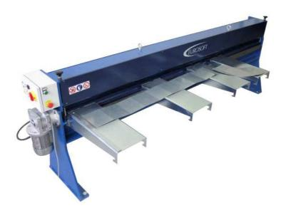
Ribbing machine for the realisation of longitudinal stiffening ribs for sheet with—thickness 1,5 mm at a speed of 20 m/minute.
