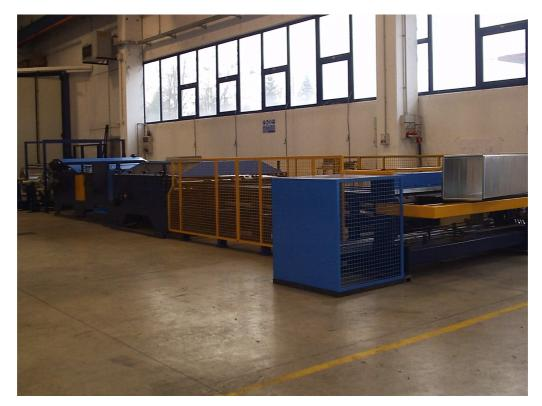
The machine consists of several modules, which are the straightener, the cutting and bending block and the profiling Pittsburgh or snapblock or both.
